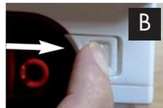
Slide the security lock of the vacuum chamber all the way to the right (picture B) and take out the vacuum chamber (picture C). Clean the vacuum chamber with a damp sponge or cloth and warm soapy water.
