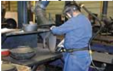
shot blasting (stage 1) and fettling
