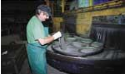
shot blasting (stage 2) and quality control check
